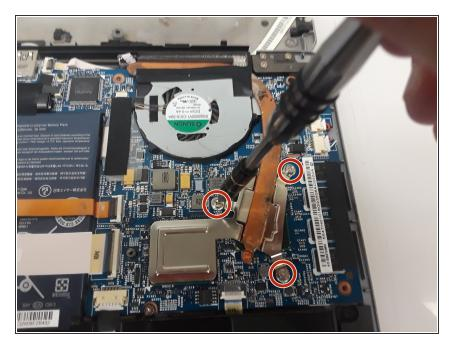
Unscrew the three screws with a Phillips #0 screwdriver.
