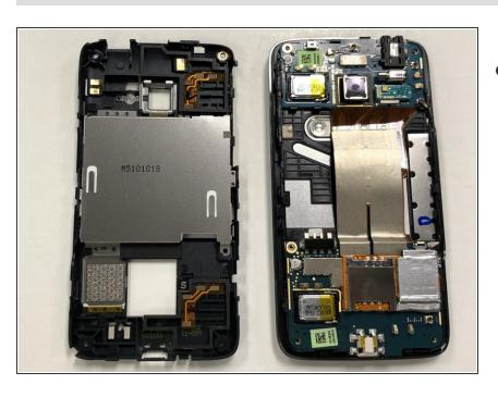
The SIM card slot will come off the device with the SD card slot and is ready to replace. To reassemble your device, follow these instructions in reverse order.
