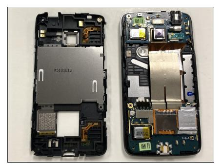
Separate the screen and back cover with the opening tool.
