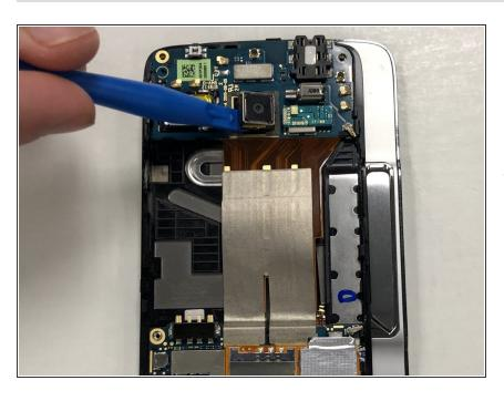
The camera is attached to the device by a sticky double-sided piece of tape. Insert the plastic
