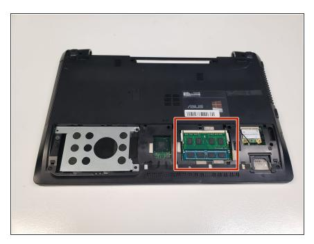
Lift the cover and locate the green and blue RAM sticks on the right side of the device.
