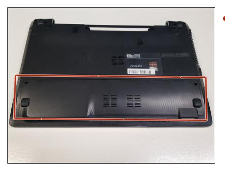
• To access the compartment that holds the RAM, flip the laptop so the bottom cover is facing upward and the battery compartment is facing away from you.
