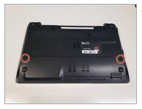
Use a Phillips #0 screwdriver to remove the two screws that hold down the compartment cover.
