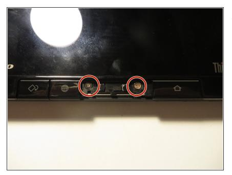
Remove the 2 screws found under the button you just removed with a size #00 Philips Head Screwdriver.
