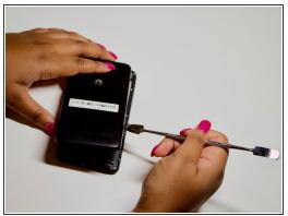
Use an Opening Tool and begin to lever up the back cover of your Huawei Pronto LTE
