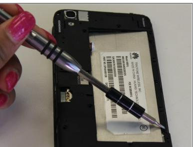
Unscrew the fifteen 0.5mm screws with a Phillips #000 screwdriver.
