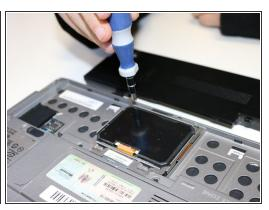
Remove the screws keeping the hard drive in place using a PH00 Philips screwdriver.
