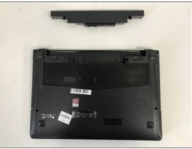
While holding the right battery lock in the unlock position, slide the battery carefully out of the laptop and set it aside.
