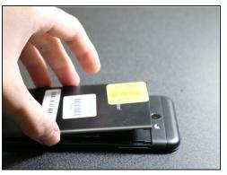
Pull up on the small indention on the right side edge and remove the back portion of the phone.
