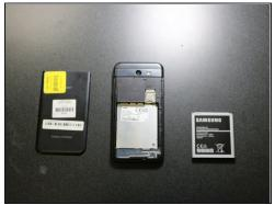
• After removing the back of the device, locate the slot below the bottom right corner of the battery and use the tip of your finger to remove it.
