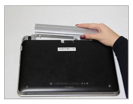
After unlocking the mechanism, slide the battery out of its compartment.
