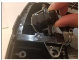
Pull out the water collector by gripping it tightly and lifting upwards.
