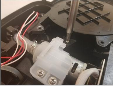
Remove the six 13.0 mm screws.
