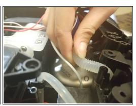
• Lift the tube, connected to the tank, off the black plastic hook and leave it off to the side of the hook.
