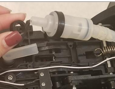
Slide the black plastic ring, which holds the puncture needle tube down, off of the tube.
