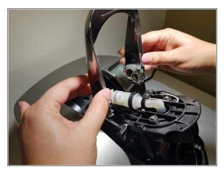
Push the handle back and upward to detach it from the Keurig.
