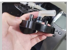
Gently pull the puncture needle down and out from the Keurig.
