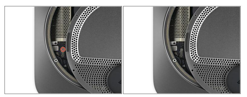
Use a T6 Torx driver to remove the 2.8 mm screw securing the antenna cable to the Mac mini's logic board.
