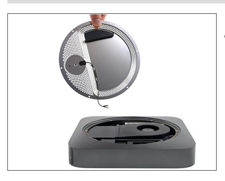
Remove the antenna plate from the Mac mini.
