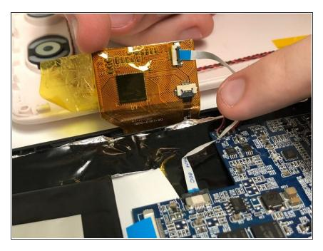
Flip up the small gate and unplug the ribbon cable shown.
