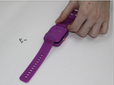
Next, use the Phillips #00 screwdriver to unscrew the four 6.0 mm screws located in each corner of the watch to remove the backplate.
