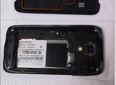
Pry the battery from the bottom of the phone to remove it.
