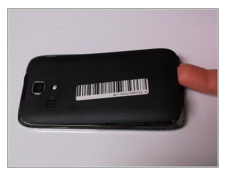
Remove the back cover by prying from the gap above the charging port.
