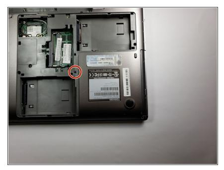
Use the Phillips head screw driver to remove the 6mm screw holding the disk drive in.
