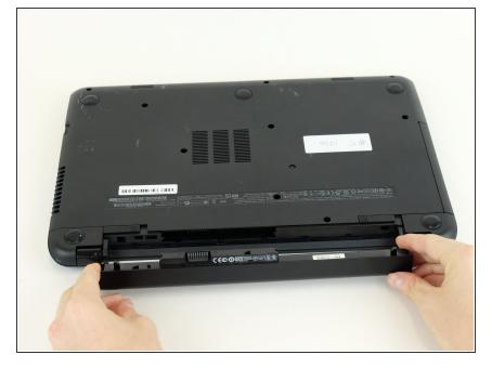
• Pull on the battery to remove.
