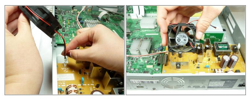
• Use your fingers to unplug the red and black wire from the yellow circuit board to completely remove the fan.
