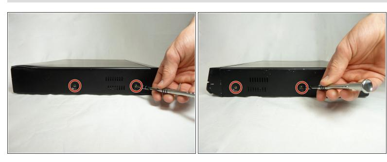
Remove the two 3mm Phillips screws on each side of the DVD player using the Phillips #1 screwdriver.
