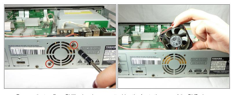
Remove the two 7mm Phillips head screws attaching the fan to the case of the DVD player.
