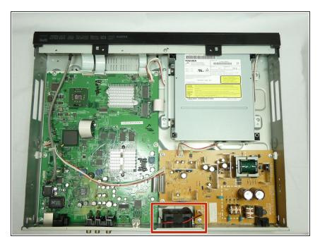
The fan will be attached to the case, connected to the yellow circuit board.
