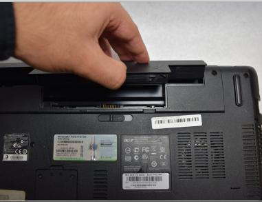
Using your fingernail, pull the battery up and out.
