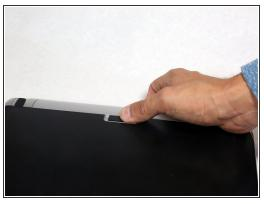
Pull the switch on the middle upper portion of laptop towards the battery symbol.
