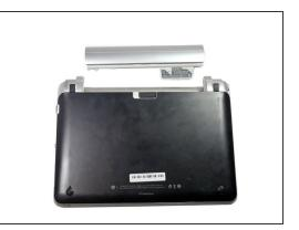
• Finally, firmly pull the battery away and outwards from the laptop.
