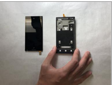
Apply heat using a heat gun or blow dryer in close proximity to the device. Then use the metal spudger to pry the display screen from the frame.
