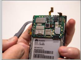
• Use a plastic spudger or your fingers to gently pry up the four flex cables from the main board.
