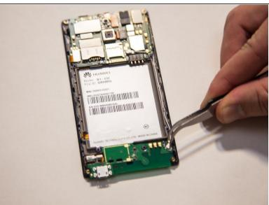
Lift gently at each connector of the white wire to disconnect the antenna from the port.
