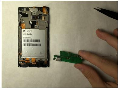
• Gently pry up near the small black clip with a plastic spudger to detach the charging board.
