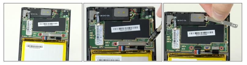
Obtain the Torx T5 screwdriver bit and ratchet from the toolkit. Locate the two 3mm black metal screws located on each side of the silver metal bracket holding the wire harness in place. Remove both screws releasing the metal bracket and set it aside.
