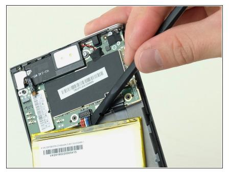
Obtain the black spudger from the toolkit and place the flat edge under the wire harness between the wires and back of the device. Gently pry upwards at an angle until the plug comes out of the harness. You may now safely remove the battery from the device.
