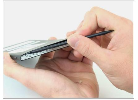
Obtain the black plastic spudger tool from the iFixit toolkit. Position the device as shown in the picture. Insert the flat end of the spudger directly in the space above the power button between the back cover and front screen.
