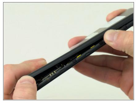
Pry around the edges of the tablet with your fingers until you have successfully removed the back of the device. Take the back cover off to access the battery.
