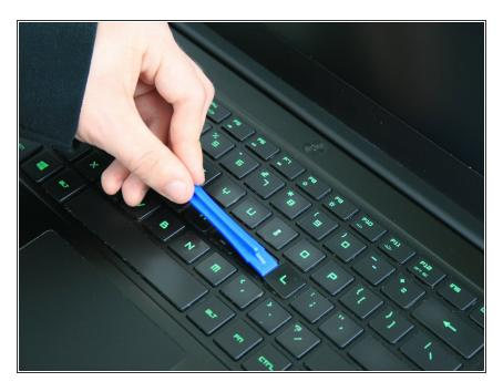
Using the opening tool insert underneath key.
