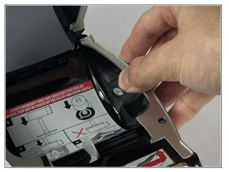
• Turn the device upright and lift the lid. Carefully pull off the side panel that has the eject button on it until the panel gives way.
