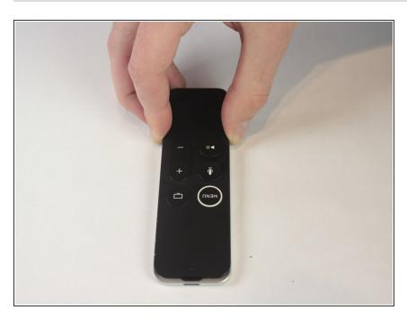
Push front face forward to disengage plastic clips at the top of the remote.
