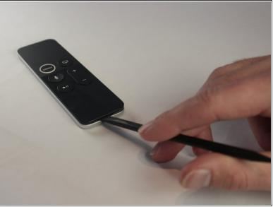
Using a spudger, gently lift the face of the remote. Starting from the bottom and working your way to the top.
