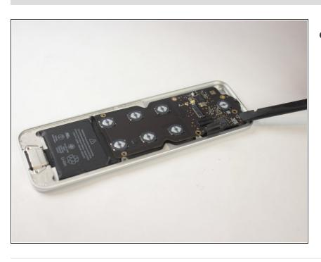
Using a plastic spudger, gently remove the logic board from the case of the remote.
