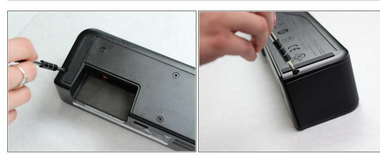
• Remove the two screws located at the outer edge of the backside with a Phillips head screwdriver.
