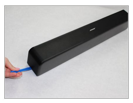
Lay the speaker on its backside with the speakers facing up. Wedge the plastic opening tool into the crack where the protective wire screen meets the housing. Pry apart until you create enough room for your fingers.
