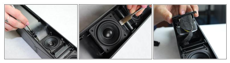
Remove the 4 screws in each corner of the speaker to remove it from the housing.
