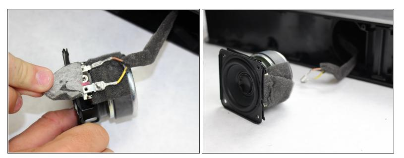
Peel back the styrofoam on the speaker & disconnect the yellow & brown wires by sliding them off the receptor.
