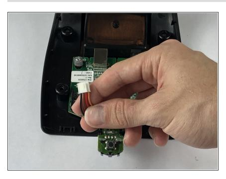
On the motherboard, unplug the power cable coming from the power button assembly.
