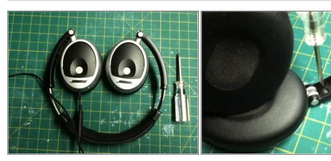
To repair a short in the wires, the head band has two screws, just above the headphones cups.
