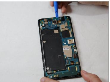
Insert and slide the plastic opening tool alongside the seam, gently wiggling the opening tool to open and remove the motherboard.
