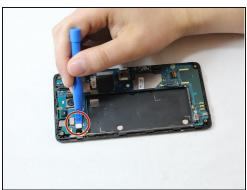
Use the plastic opening tool to unplug the three connectors.
