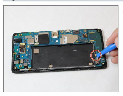
Use the plastic opening tool to push up on the wire to remove it completely.
