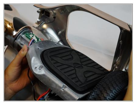
Separate the upper shell of the hoverboard and the metal layer inside.
