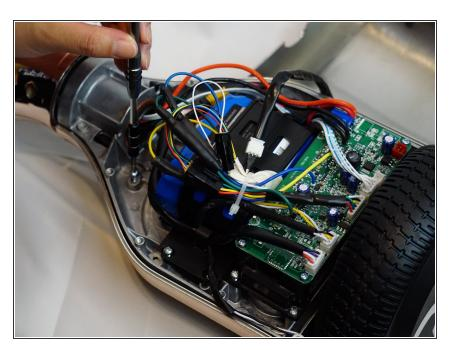
Remove the screws from the metal layer inside the hoverboard using a Phillips #1 screwdriver.
