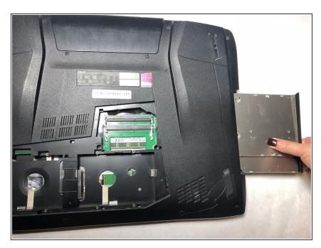
Pull out the optical drive to revel the screws holding the laptop cover.
