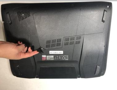
Lift up the rubber tab located in the upper-right corner of the backing plate.
