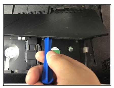
Carefully pull the backing plate off. If you have a pry tool, you can pry on the edges carefully.
