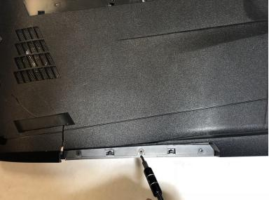
Remove all 10 5.2mm Phillips screws holding the main back cover using the Phillips #1 screwdriver.
