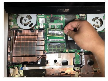
Carefully, pull on the side tabs to release the RAM card.
