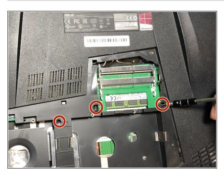
Remove the four 5.2mm screws directly behind the backing plate using the Phillips #1 screwdriver.
