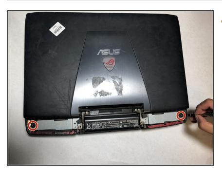
Remove the two 6.8mm Phillips screws directly below the vent covers using the Phillips #1 screwdriver.
