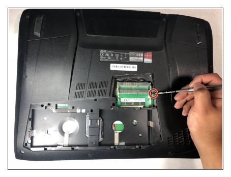
Use a Phillips #1 screwdriver to remove the 5mm screw on the right side.
