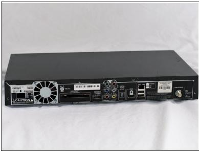
• Remove the four 80 mm T10 screws from the back of the TiVo box using the Torx screwdriver.
