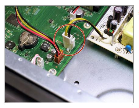
Remove the power cable from the motherboard by gently pinching the connector.
