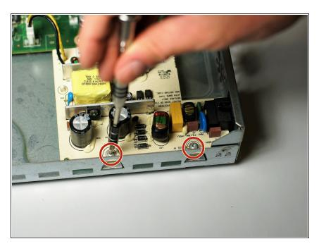
Remove the two 80 mm T10 screws from the power supply using a Torx screwdriver.
