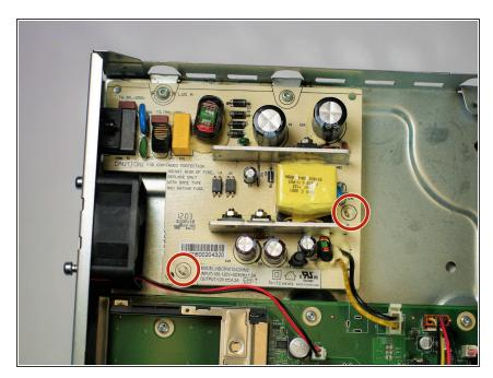
Pinch the two plastic plugs and lift the power supply to detach the plugs from the board.
