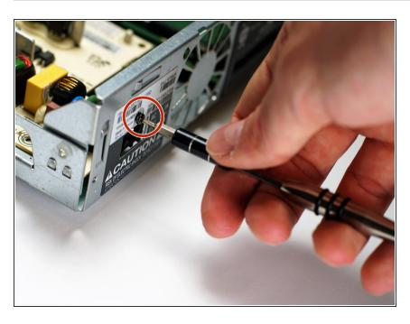
Remove the 140 mm T8 screw from the back of the TiVo premiere XL4 box holding the power supply in place using a Torx screwdriver.
