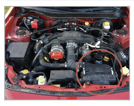
Locate the air filter box, which can be found to the front right of the car.
