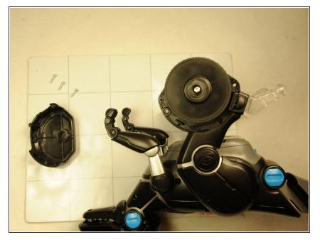
Remove the 1.2 mm Phillips screws surrounding the wheel and take off the wheel cover.
