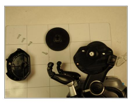
Remove 1.2 mm Phillips screw from the white plastic piece in the center of the wheel and then remove the wheel entirely.
