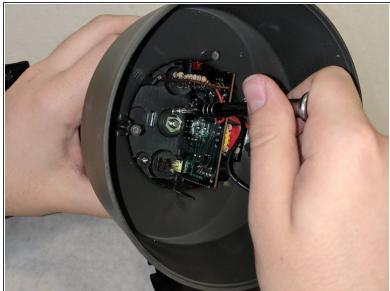
Unscrew the single 1.2 mm Phillips #1 screw holding the motherboard to the plastic lantern housing.
