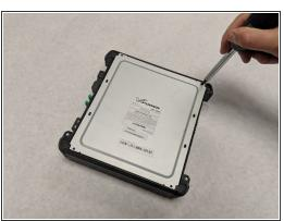
Remove all the Phillips 10.0mm and 7.0mm screws on the outside of the case.
