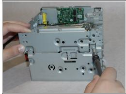
Remove the four 5.5mm screws with the Phillips #1 screwdriver.
