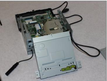
• Flip up the black clasp with a spudger to disconnect the large white ribbon cable connecting the CD drive to the board underneath.
