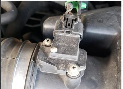
Connect the wiring harness back on the sensor.
