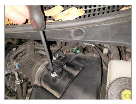
Insert the new sensor and secure it down using the Philips screwdriver.
