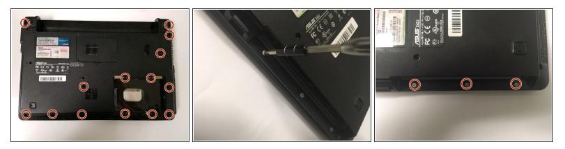
• Remove all screws located on the bottom plate of the laptop, beginning with the three located underneath the disc drive.
