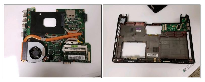
• Remove the motherboard from the device.
