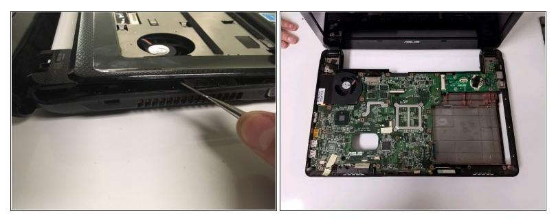
• Pull up on the front panel using the <u>spudger</u> until the front panel separates from the bottom panel.
