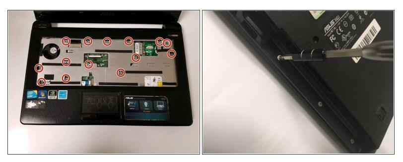
Rotate the laptop until it is sitting face up and extract all screws exposed by removing the keyboard.
