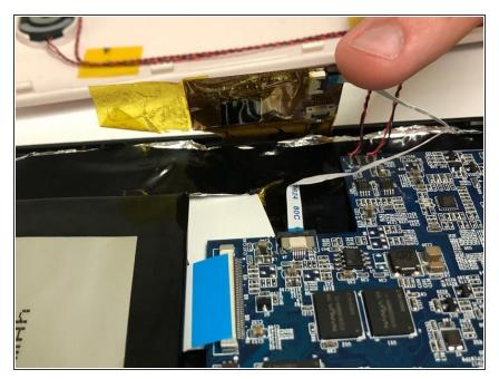
Peel back the touch interface chip (which is on the top right of the motherboard, covered in yellow tape.)
