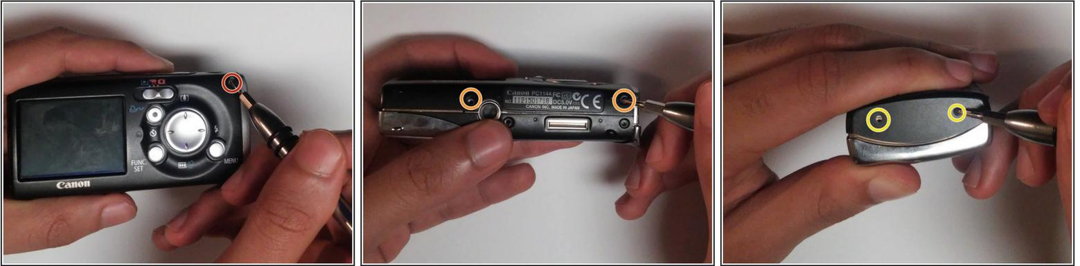
**i** Remove the wrist strap and battery before removing the back cover.
