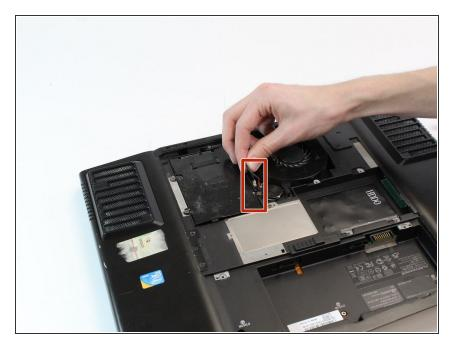
Gently pull on the coin cell battery cable to disconnect it from the laptop.
