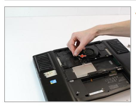
Pull on the battery to remove.
