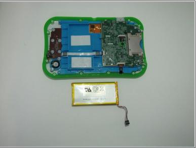
Carefully remove the battery from the LeapPad, use the plastic spudger to gain leverage, if needed.
