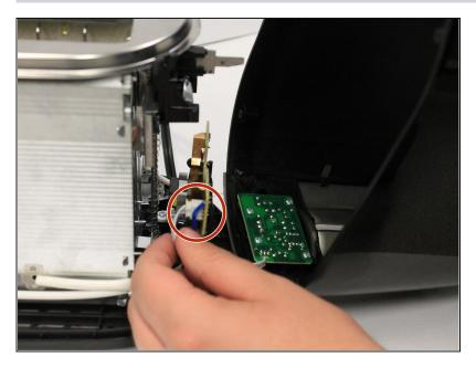
Detach the bundled cable connector by carefully pulling it away from the circuit board.
