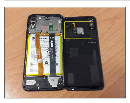
Release the ZIF connector to remove the Fingerprint scanner cable from the back cover.
