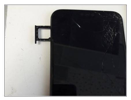
Turn the phone off and remove the SIM Tray before beginning the repair
