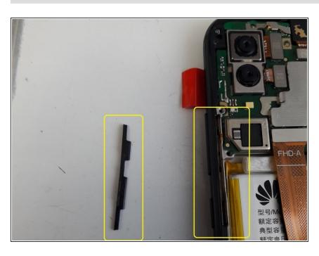
On the left side in the frame, is a small plastic retainer. Remove this and transfer to the new frame.
