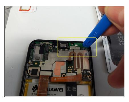
Using a spudger, carefully pry the mainboard up on the upper right corner to release it from the frame.
