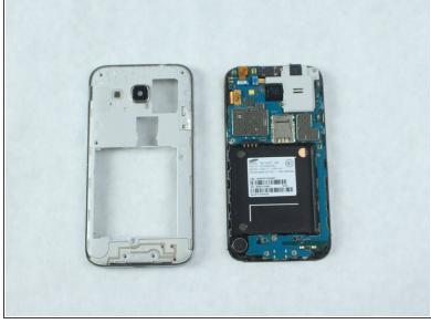
• Use an <u>iFixit Opening Tool</u> or a similarly shaped tool like a guitar pick to lift the mid-frame.
