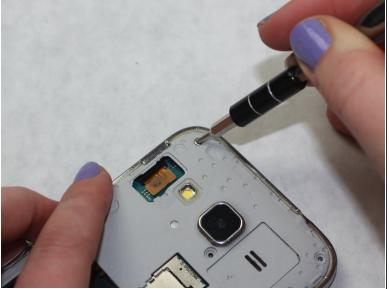
• Use a Phillips #00 screwdriver to remove the eight 4mm screws from the midframe.
