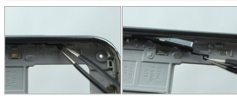
Use tweezers to unhook both of the rubber fixtures holding the volume button to the frame.
