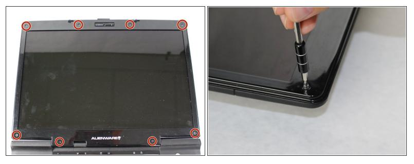
Remove the eight 7 mm screws around the edge of the screen using a Phillips #1 screwdriver.
