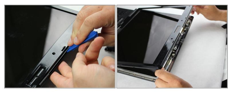
Insert the plastic opening tool and gently slide it around the edge of the screen to lift the face of the screen away from its base.
