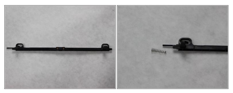
• If the spring is defective, slide it off the end of the assembly and replace it.
