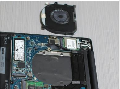
With the screws removed, lift up on the fan and remove it from the laptop.
